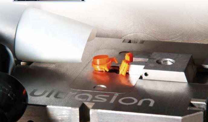
The technology uses standard room temperature pellets which as they are melted and injected in one process eliminates residence time and therefore eliminates material degradation.
